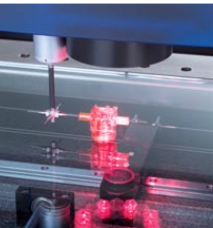
Precise: The optical sensor on O-INSPECT is particularly well-suited to monitor small, complex parts.
